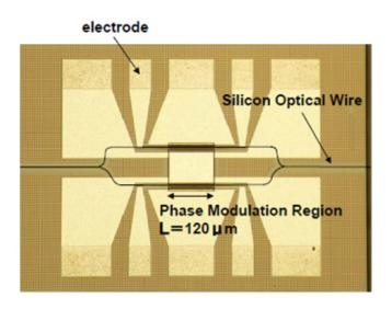
**Tokyo, March 23, 2010** - NEC Corporation (NEC; TSE: 6701), announced today the successful development of a silicon MOS (metal-oxide-semiconductor) optical modulator that boasts a leading power-consumption efficiency of less than 1mW/Gbps, a compact size of 120 μm in length and high-speed operation of 25Gbps. The device has only one-tenth the power consumption when compared to conventional PN-type silicon optical modulators.
